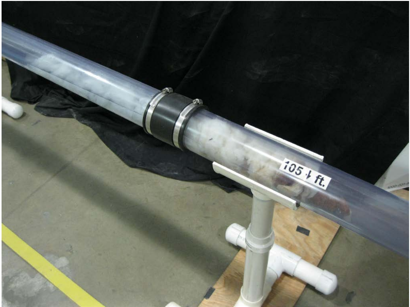
Photo 4-1, Paper Accumulation Resulting in Full Pipe Condition, 3.8 Lpf / 1.0 gpf Flush Volume Test Run, 3-inch Diameter Apparatus
